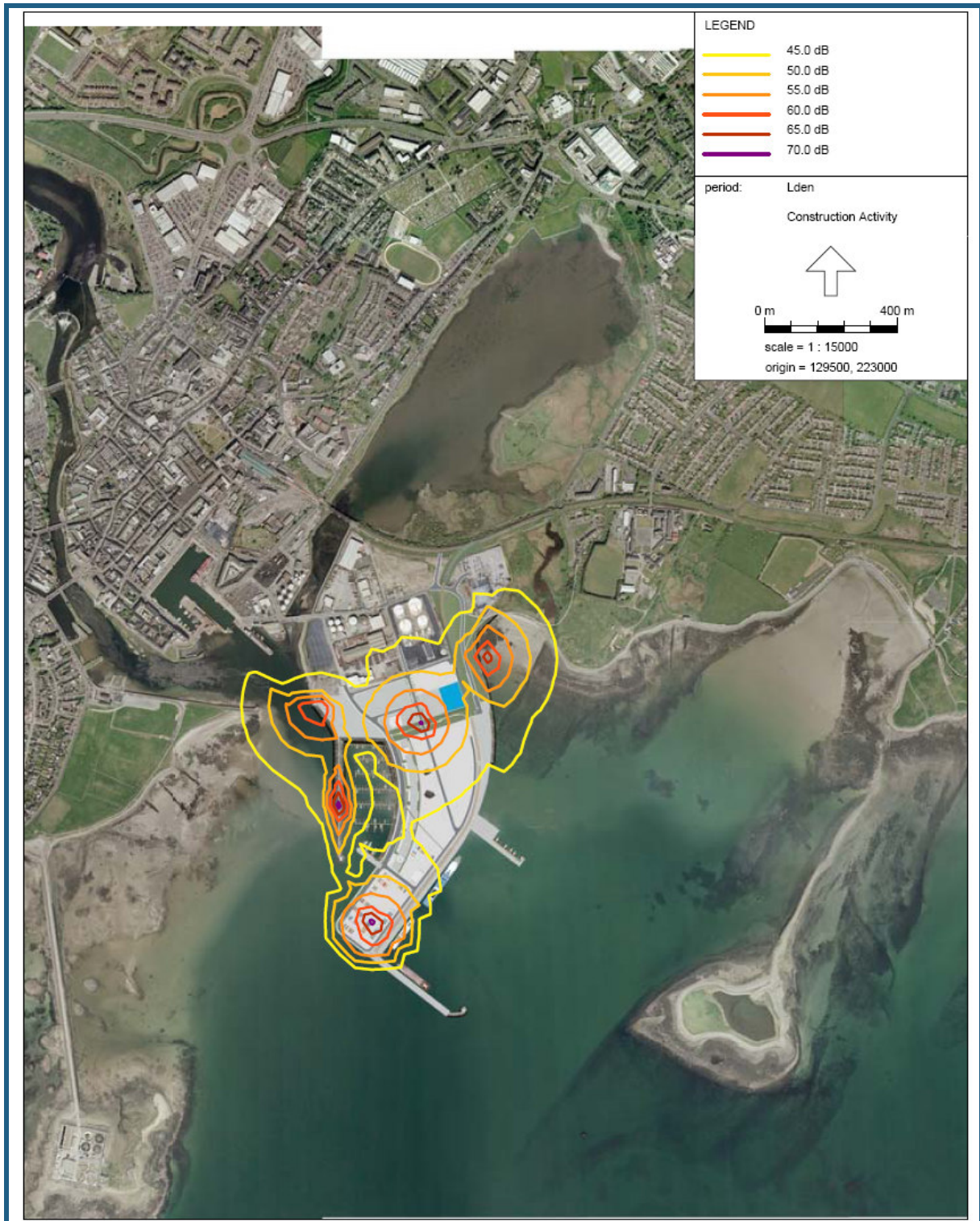
Figure 10.4.1 - Lagoon Construction Noise Model
